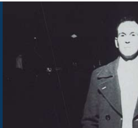
Conventional IR Illuminator, hot spot in foreground, poorly illuminated background
